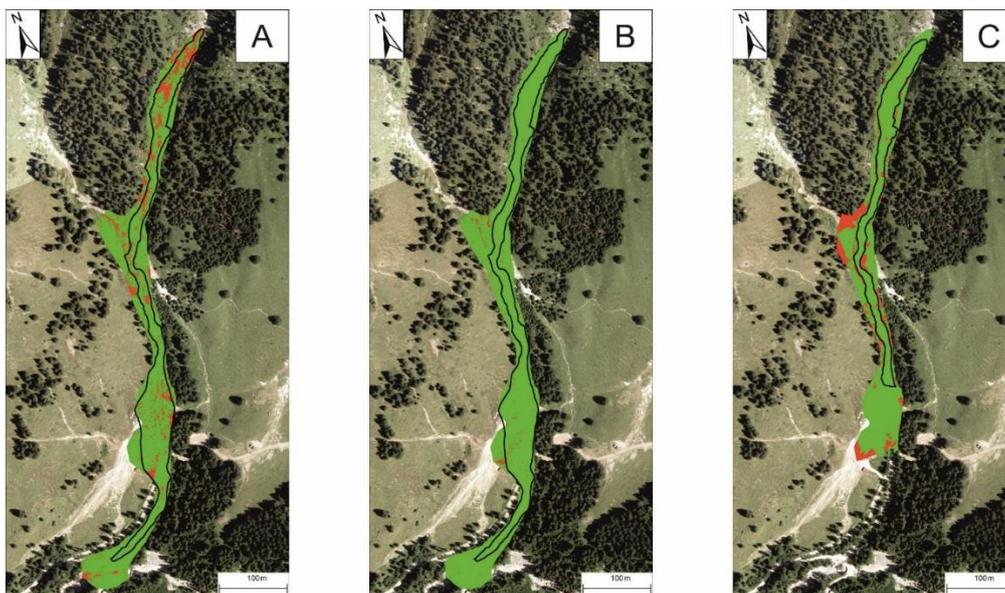
Fig. 4. Due to occlusion the generated DEMs have areas without data (red) that have to be interpolated in order to calculate geomorphic changes. A: TLS of June 2015; B: TLS of June 2017; C: UAV of July 2017. Black outline: Area of interest. Orthophoto provided by Bavarian Land Surveying Office
