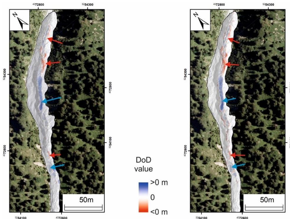
Fig. 5. DoDs derived with SfM-MVS (left) and TLS (right) between May and July 2017. Orthophoto provided by Bavarian Land Surveying Office
