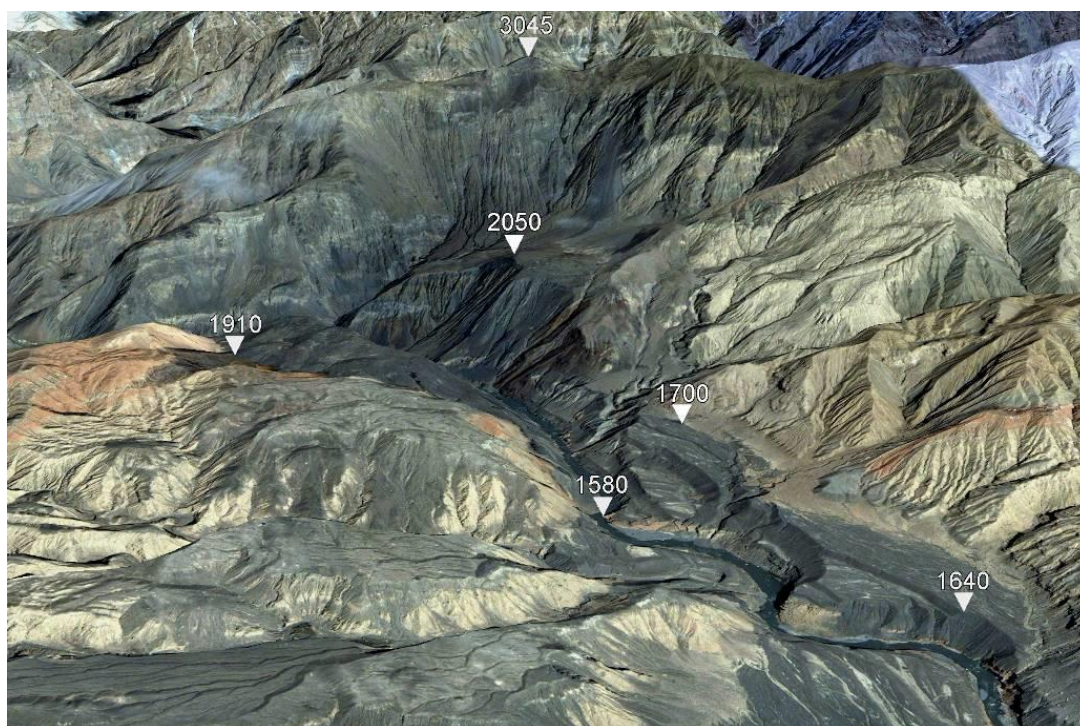
Fig. 11. Evidence of the catastrophic outburst flood caused by the Sarydjaz-Aksu rockslide dam breach – terraces up to 120 m high "painted" by dark-grey debris eroded from the dam's body. 3D Google Earth view
