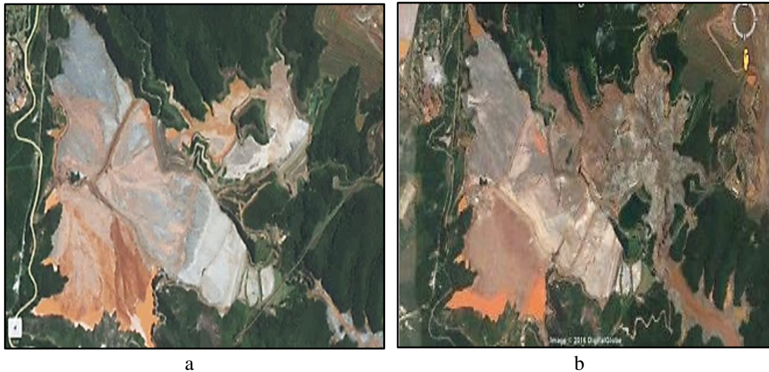
Fig. 1. Fundão Dam and Reservoir; (a) during construction and before rupture, and (b) after rupture and upon emptying of the reservoir
