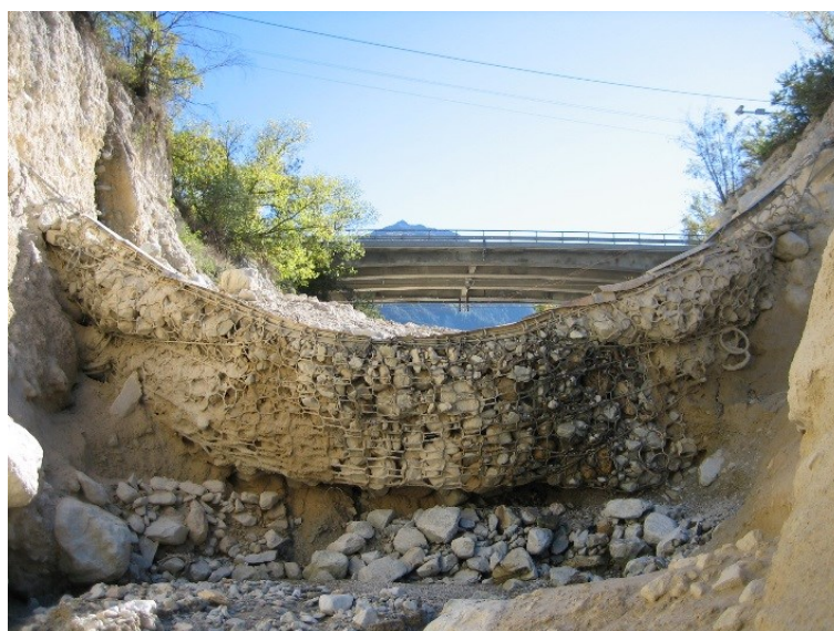
Fig. 1. Testing of debris flow retention system with ring net in the Illgraben channel, 2006. Retention volume approx. 1000 m 3
