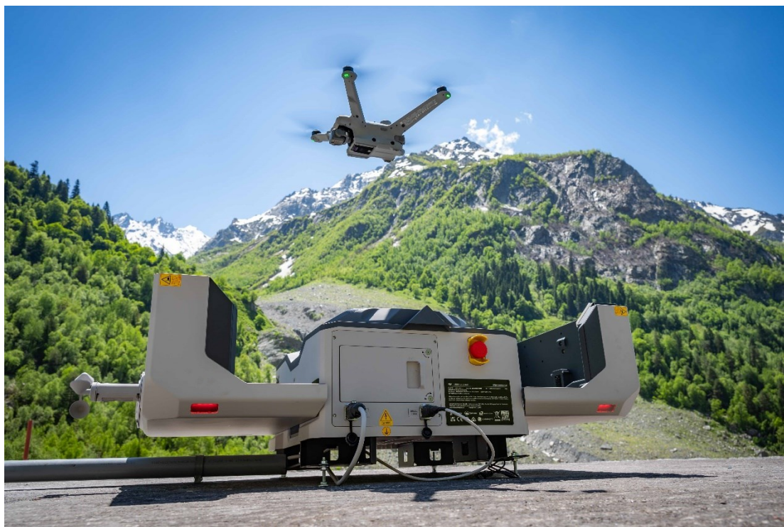
Fig. 7. DJI drone dock 2 taking off from the intake building of Mestiachala HPP
