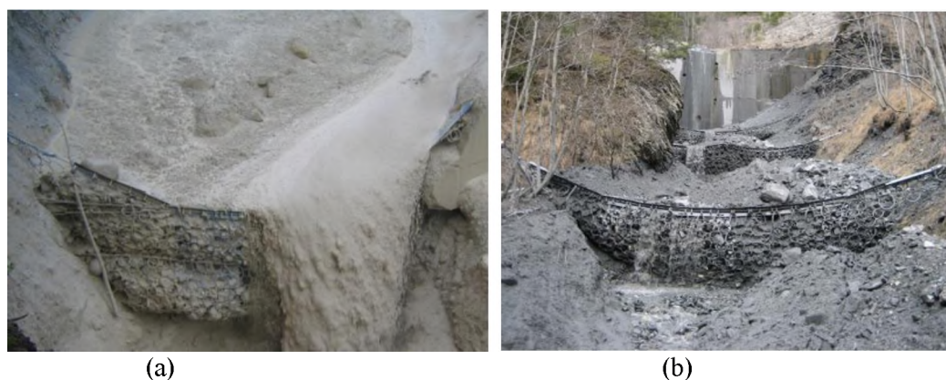
Fig. 2. (a): flexible ring net barrier withstanding overflow in the Illgraben; (b): 1:1 field testing of multi-level barriers in Merdenson, Valais, Switzerland
